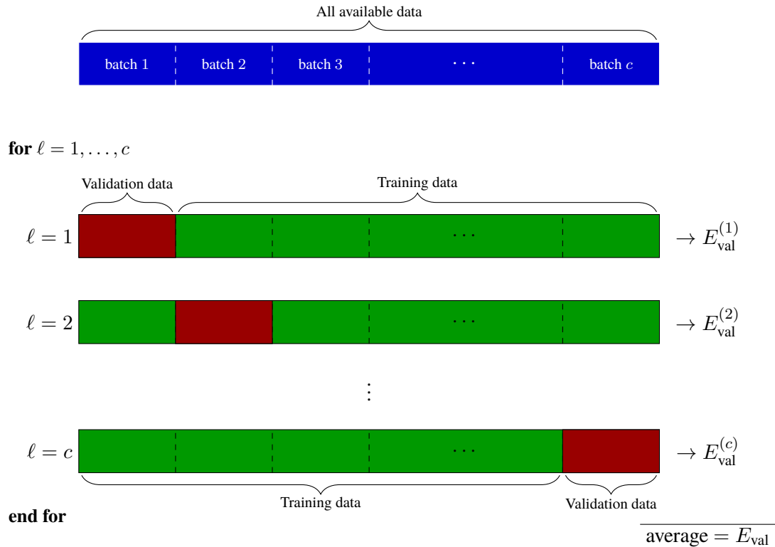
Figure 5.2: Illustration of c -fold cross-validation. The data is split in c batches of similar sizes. When looping over \ell = 1, 2, \dots, c , batch \ell is held out as validation data, and the model is trained on the remaining c - 1 data batches. Each time, the trained model is used to compute the average error E_{\text{val}}^{(\ell)} for the validation data. The final model is trained using all available data, and the estimate of E_{\text{new}} for that model is E_{\text{val}} , the average of all E_{\text{val}}^{(\ell)} .
