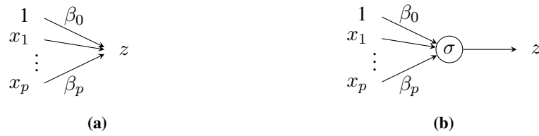
Figure 7.1: Graphical illustration of a linear regression model (Figure 7.1a), and a generalized linear regression model (Figure 7.1b). In Figure 7.1a, the output z is described as the sum of all terms \beta_0 and \{\beta_j x_j\}_{j=1}^p , as in (7.3). In Figure 7.1b, the circle denotes addition and also transformation through the activation function \sigma , as in (7.4).
